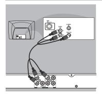
Use the composite video cable (yellow) to connect the DVD player's VIDEO(CVBS) jack to the video input jack(or labeled as A/V in,Video In or Composite) on the TV(cable supplied). To hear the sound of this DVD player through your TV, use the audio cables(white/red)to connect AUDIO OUT(L/R)jacks of the DVD player to corresponding AUDIO IN jacks on the TV(cable supplied).
